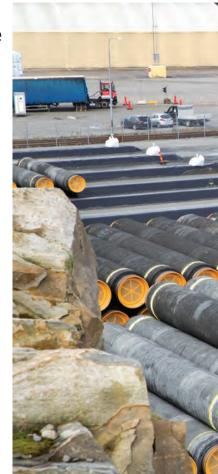
Length 12 metres, weight 20 tonnes, diameter 1.2 metres – 52,000 such pipes will come to the Port of Karlshamn where they are unloaded and stored to then be shipped out to the laying vessel once laying begins.
